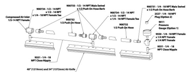
Pipe thread sealant should be applied to all threads (small packet included). Avoid the inside diameter of the fitting so it does not enter into the Air Knife.
