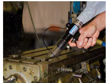
The Model 6194 Deep Hole Vac-u-Gun cleans the t-slots on a milling machine.
